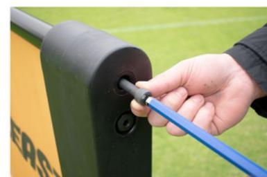
**6** Screw the top bolt using a 10mm hex key
