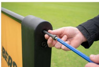
**1** Unscrew the top bolt using a 10mm hex key
